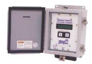
Corrosion rate measurements are made using the linear polarization resistance technique. The instrument measures the current required to polarize
